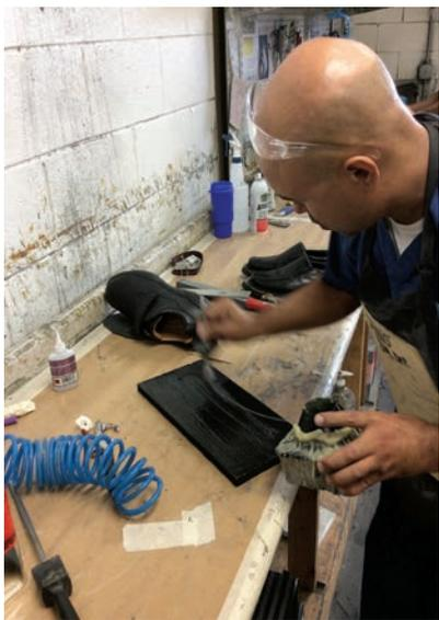
with. This is especially important when bonding two materials, such as the shoe and the EVA in this case, as these different materials adhere best when heated. Chino takes the shoe and EVA out of the oven and glues them together.
