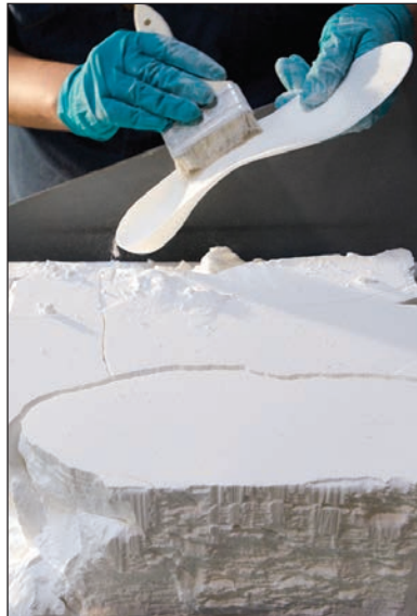
The SOLS SLS 3D Printing Process
