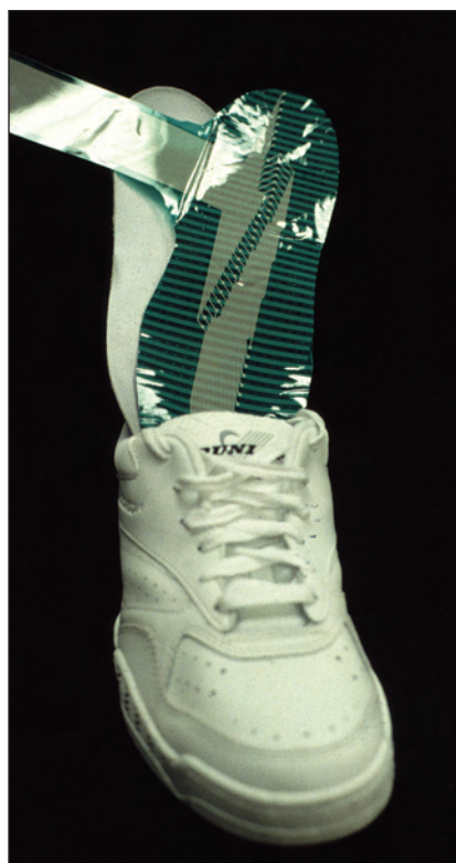
Figure 1a. F-Scan insole sensor being placed in an athletic shoe with the manufacturer's supplied shoe sock liner.
