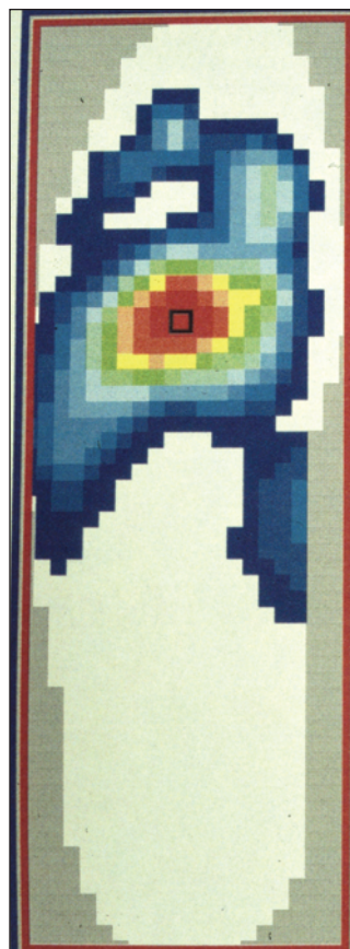
Figure 1b. F-Scan recording using the shoe alone, demonstrating high pressure areas under metatarsal heads
