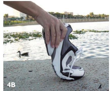
Figures 4 A, B: Forefoot flexional stability—Forefoot flexibility depends on both durometer of the midsole material and the depth of the flex grooves. Deeper grooves allow more flexibility of the shoe at the forefoot. The shoe should flex at the metatarsal-phalangeal joint, not further proximal through the midfoot.
