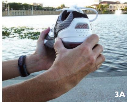
Figures 3 A, B: Midfoot torsional stability (shank rigidity)—Twist the shoe while grasping the heel and forefoot to determine the amount of stability or flexibility. Midfoot rigidity is necessary for running footwear.
