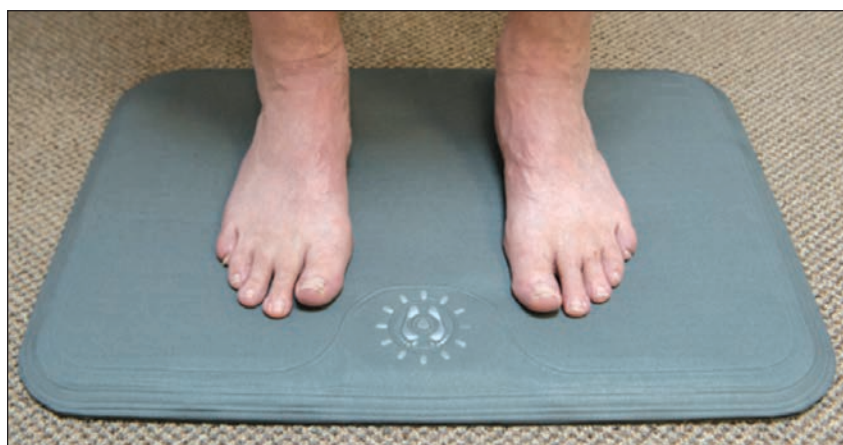
Figure 5: The Podimetrics Mat™ a thermometric mat designed for easy in-home use to monitor asymmetric skin temperature, which correlates to foot disease. R. G Frykberg, 2017(25)
